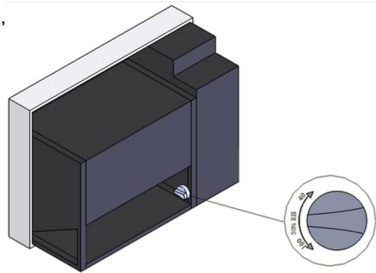
**Constant measure of the humidity** Dantherm recommends that an external hygrostat is installed to ensure a constant measure of the humidity in the pool area.
